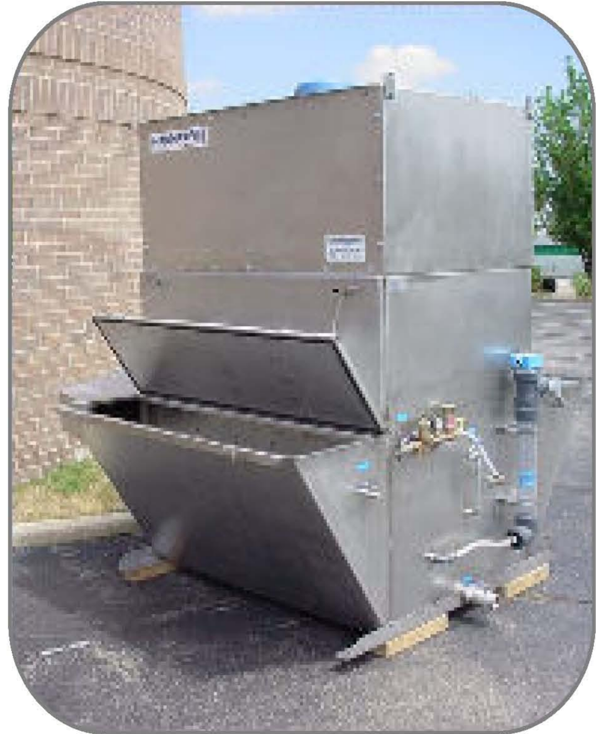
Top Picture showing Air Canada double sided Wet Collector Scrubber with tub door open and the full Electronic Automatic Water Level Control System. Control Panel remote mounted.
