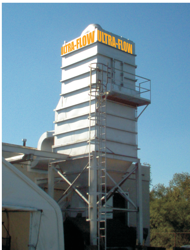
BV Series bag house at 15:1 filter ratio, collecting fine carbon dust, no after-filter, recirculating clean air back into the plant.
